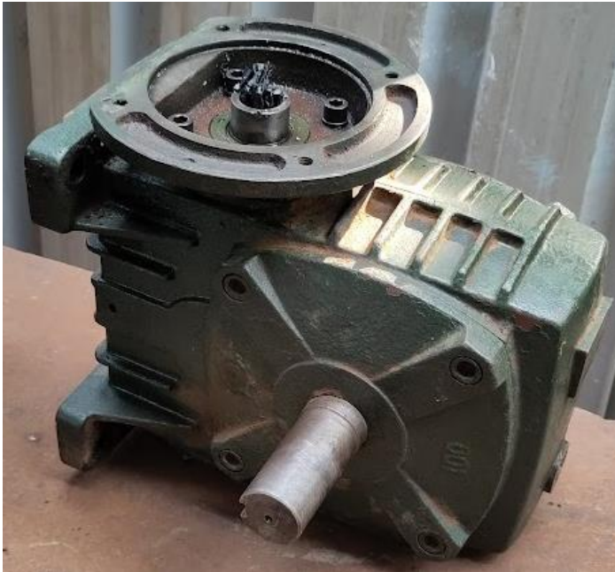
Figure 6: Image shows the initial reduction gear.
