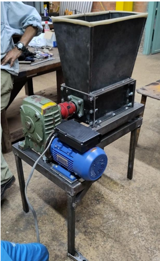
Figure 4: Complete assembly of first shredder. Motor (blue), reduction gear (green), coupling (red), shredder box (black) and hopper (black top) make up the total assembly, mounted to a frame.
