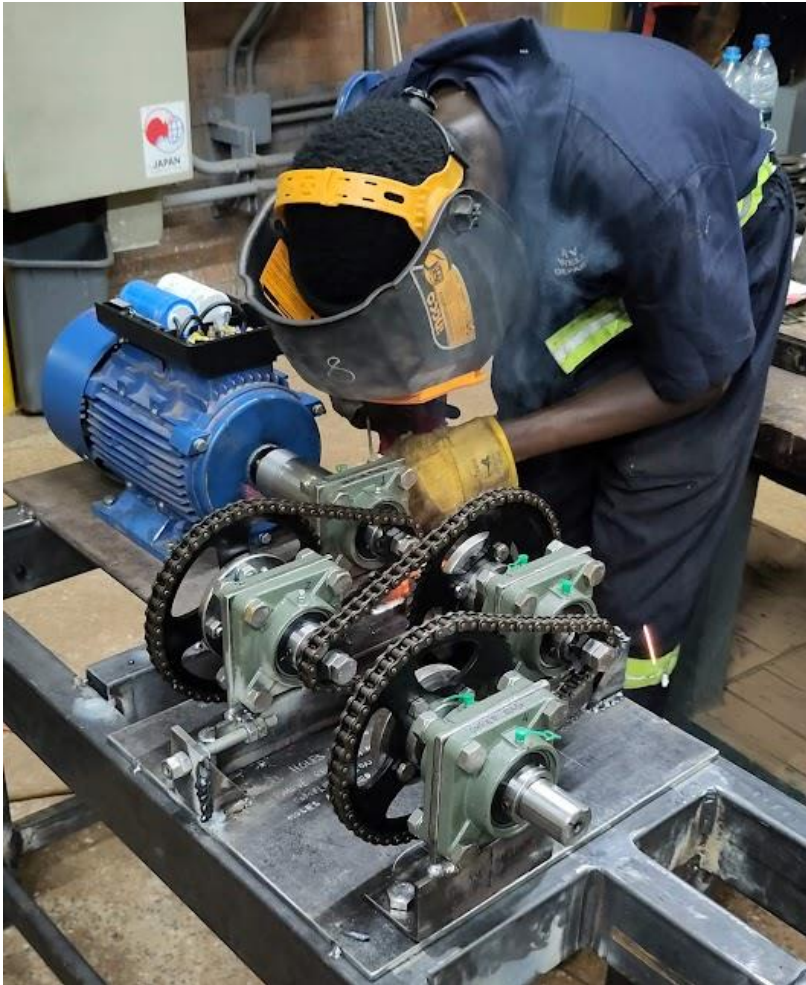
Figure 7: Finished reduction gear is being welded to the frame for function testing. The coupling to the motor was made at Nakawa to fit the shaft dimension.
