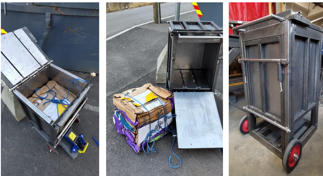
Figure 8: First baler prototype and testing
