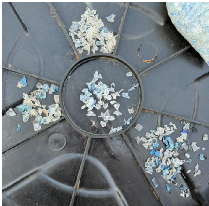
Figure 15: Shredded plastic sample, unwashed and washed. This sample is from before upgrading the shredders with new motors.
