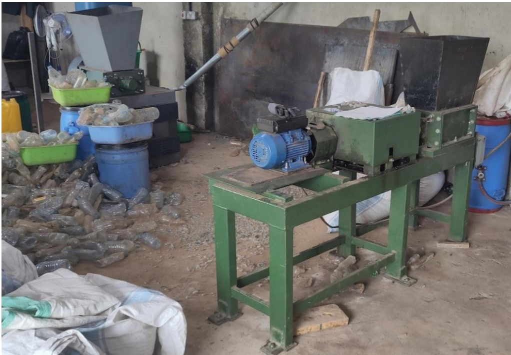
Figure 5: Complete set-up of second (right) and third (left) shredder. The reduction gear (green box) has been replaced on the second shredder.
