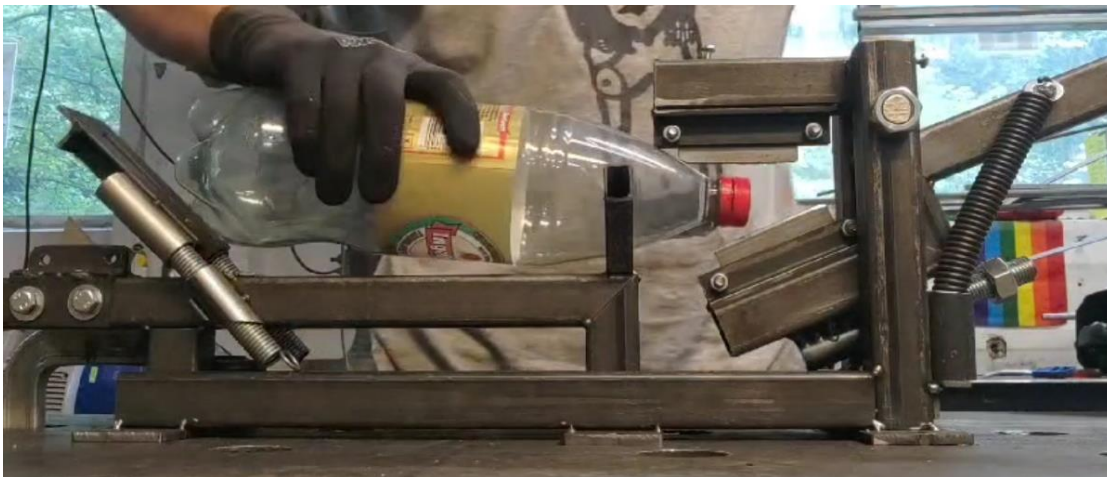
Figure 11: Bottle cutter testing
