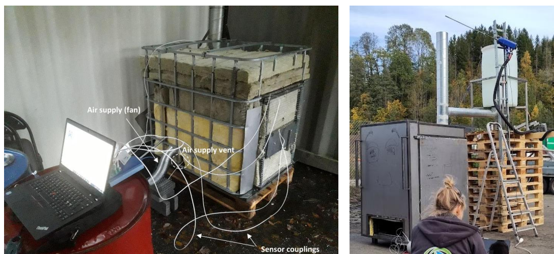
Figure 3: First (left) and second (right) pyrolysis unit being tested
