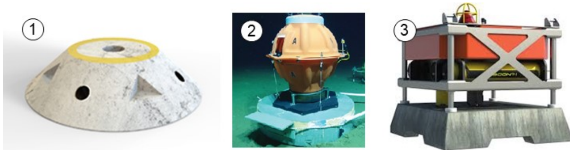
Figure 4.18 From left to right 1) Concrete benchmarks used by Quadgeo for gravimetric surveys, 2) Sonardynes FETCH instrument node on concrete benchmark deployed by Scripps for monitoring tectonic motion in the Cascadian subduction zone (photo David Chadwell) and 3) Concrete foundation block for Kongsberg's K-lander
