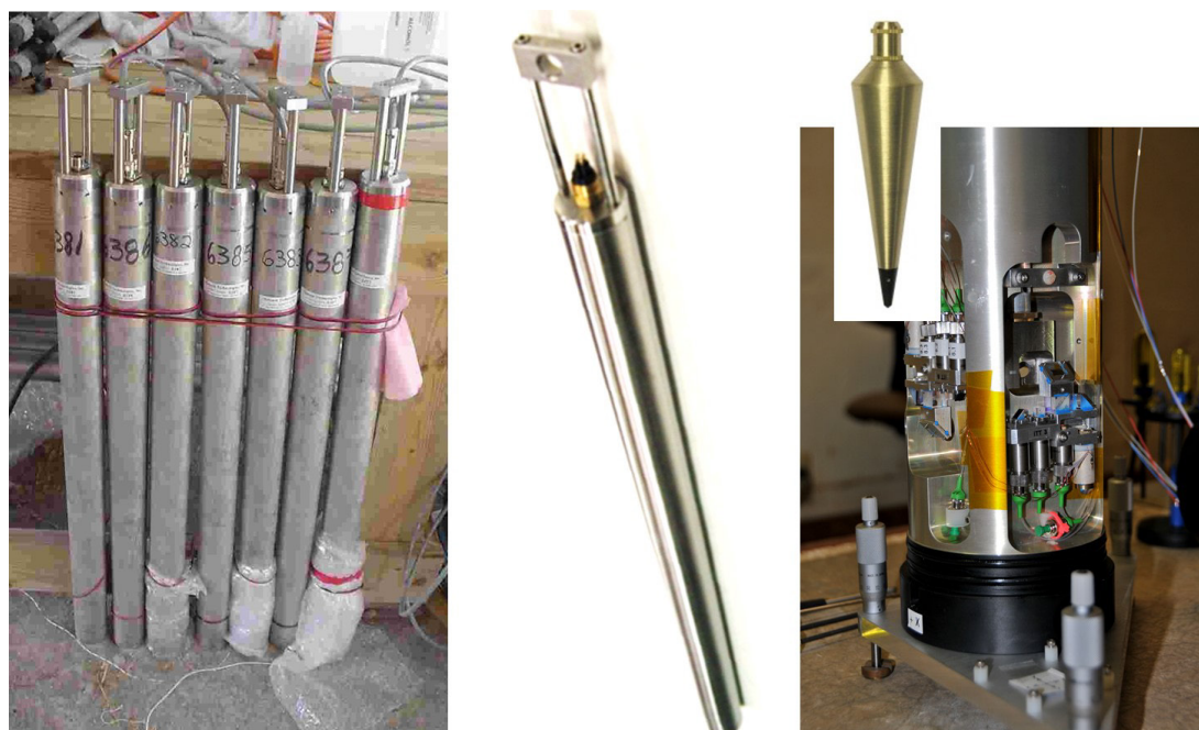
Figure 4.16 Precision downhole inclinometers from Pinnacle (Halliburton) and Jewel instruments usually installed to monitor fracking. Right: Optical pendulum type of inclinometer from Scripps
