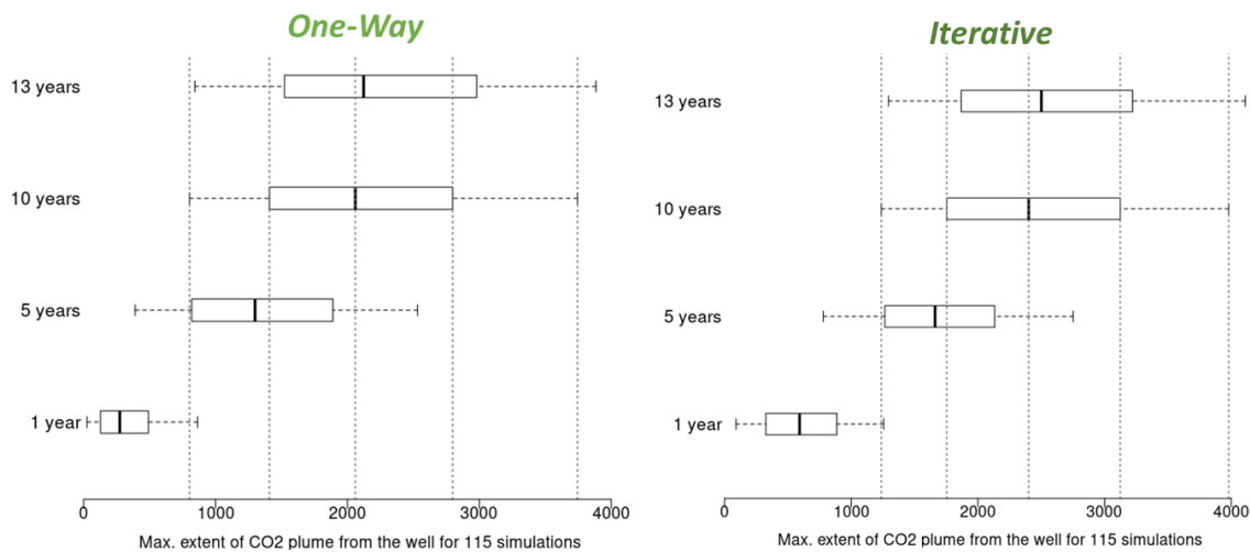
Figure 44 : Box plots (describe results distribution with the median (bold line), percentiles 25 and 75 % (box) and dispersion (segments)) of the maximum extent of CO 2 plume for 115 simulations for several injection periods (1 year, 5 years, 10 years) or post-injection (13 years) at the top of storage formation.
