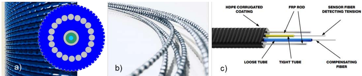
Figure 2. Example of engineered cables for DSS ground deformation monitoring; a) Solifos V3 grip armoured cable; b) Epsilon composite DSS cable with 4% strain range from Nerve sensors and c) DSST cable from Fibrain
